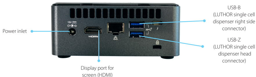
Figure 7. NUC rear panel ports.
