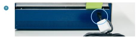
Insert the CAB2 (mini PC (NUC) power cord) into the power inlet on the rear of the mini PC (NUC), and then insert the other end of the power cord into a properly grounded wall outlet or UPS.
