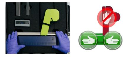
Remove the black protective foam around the pipetting head. Then remove the strap that holds the USB cable on the right side of the LUTHOR single cell dispenser.
